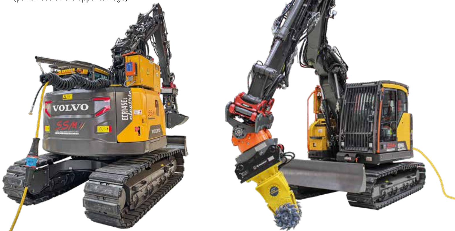
ECR145E with electric drive and radio remote control (power feed on the upper carriage)
