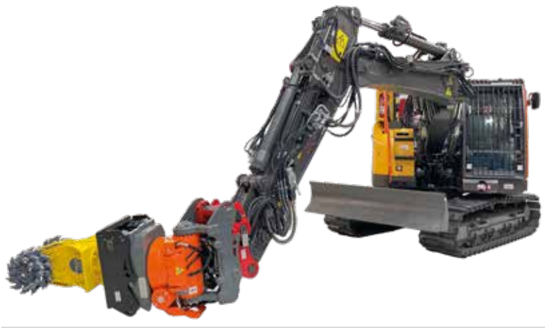
Laterally adjustable offset-boom
