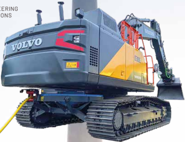
EC300E with dual drive (cable reel at the undercarriage)
