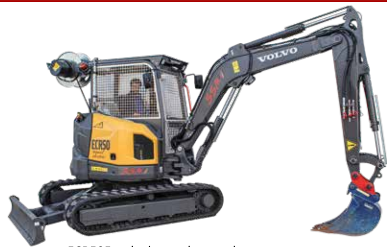
ECR50F with electric drive and radio remote control
