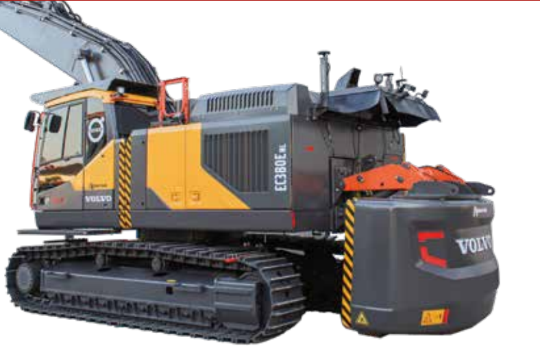
Hydraulically detachable rear counterweight
